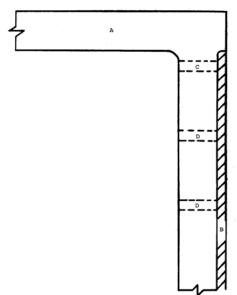
6. When friction welding is used to attach plastic components, all deformed material shall be removed to eliminate any cracks, crevices, pits or folds. No radius is required at these junctures.
