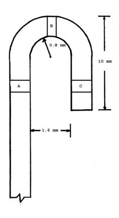
Figure I.2 Perforations in a formed stiffening rim on the top of a metal cheese mold is required at one or more of locations A, B, or C to facilitate cleaning.
