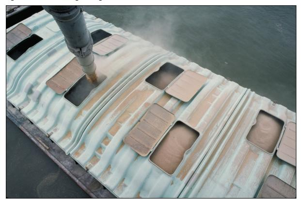
Figure 12-5: Grain barge being loaded.
