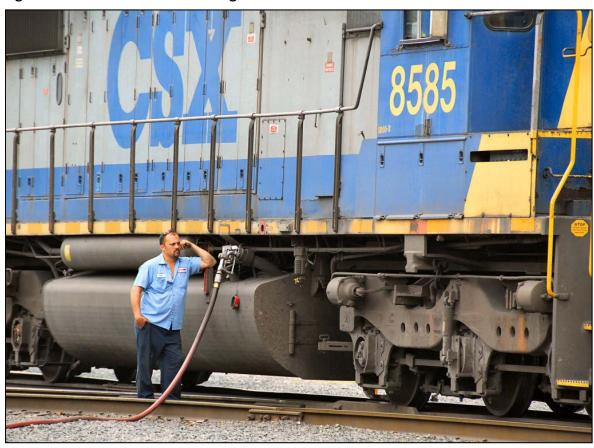
Figure 15-9: A locomotive refueling
