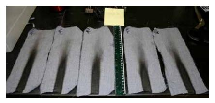
optimum flame resistance performance. 34 blend samples in a woven construction were produced and evaluated for flame resistance and mechanical properties. From this analysis 7 blends are selected and spinning of yarns has commenced.
