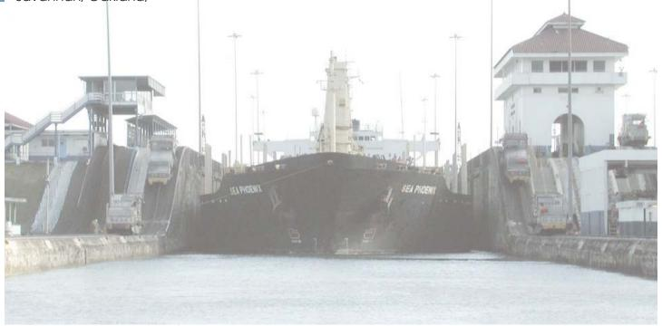
1 Post-Panamax containerships usually move about 5,000 - 8,000 containers, have widths of 14 to 20 containers, and drafts of 15 meters, requiring an access channel of 17 meters deep. Super Post-Panamax vessels have a carrying capacity greater than 9,000 containers. (Knight 2008)
