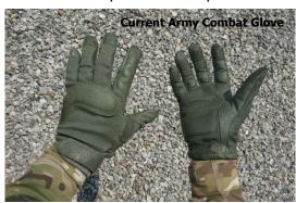
The Army Combat Glove (ACG) is a critical part of a soldier's combat gear, providing important protection in combat operations. It is important that the ACG meet flame resistance properties in order to protect soldiers' hands from flame and blast threats. At the same time, it is highly important that the ACG provide comfort and durability in typical environmental conditions experienced in combat. Program Manager Soldier Combat Individual Equipment (PM SCIE),
